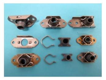
These are great! If you damage the threads, all you have to do is squeeze the retaining spring with needle nose pliers, remove the damaged nut insert, and replace it with a new insert. These Self Locking Nut Plates, floating, variable counter bore, with replacement nut element; come in both 450 DEG F and 800 DEG F types and are available in 2 lug and 1 lug configuration.
